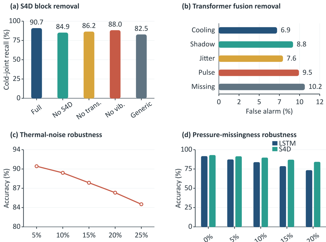
Figure 6. Ablation and robustness analysis. (a) S4D block removal. (b) Transformer fusion removal. (c) Thermal-noise robustness. (d) Pressure-missingness robustness.
