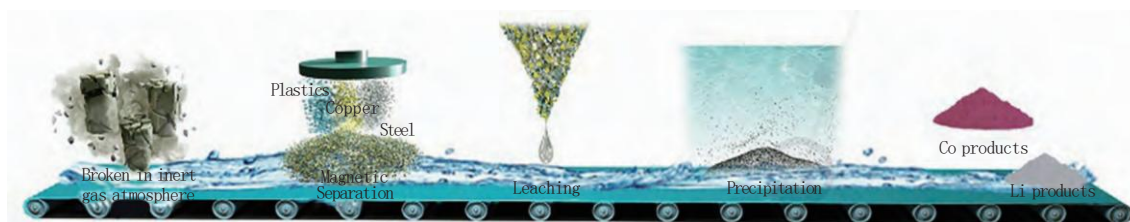
Figure 8 Schematic diagram of hydrometallurgy
