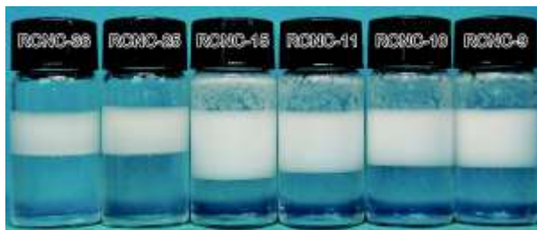
Figure 4 Optical image of an O/W Pickering emulsion prepared with 2 g/L RCNC-n
