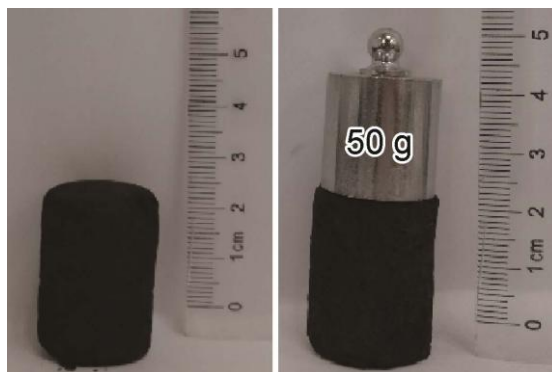
Figure 6 Load-bearing abilities of CdS/rGO composite aerogel.
