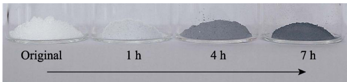
Figure 4 Color variation of \text{TiO}_{2-x} prepared by ultrasonic synthesis method with time [46]
