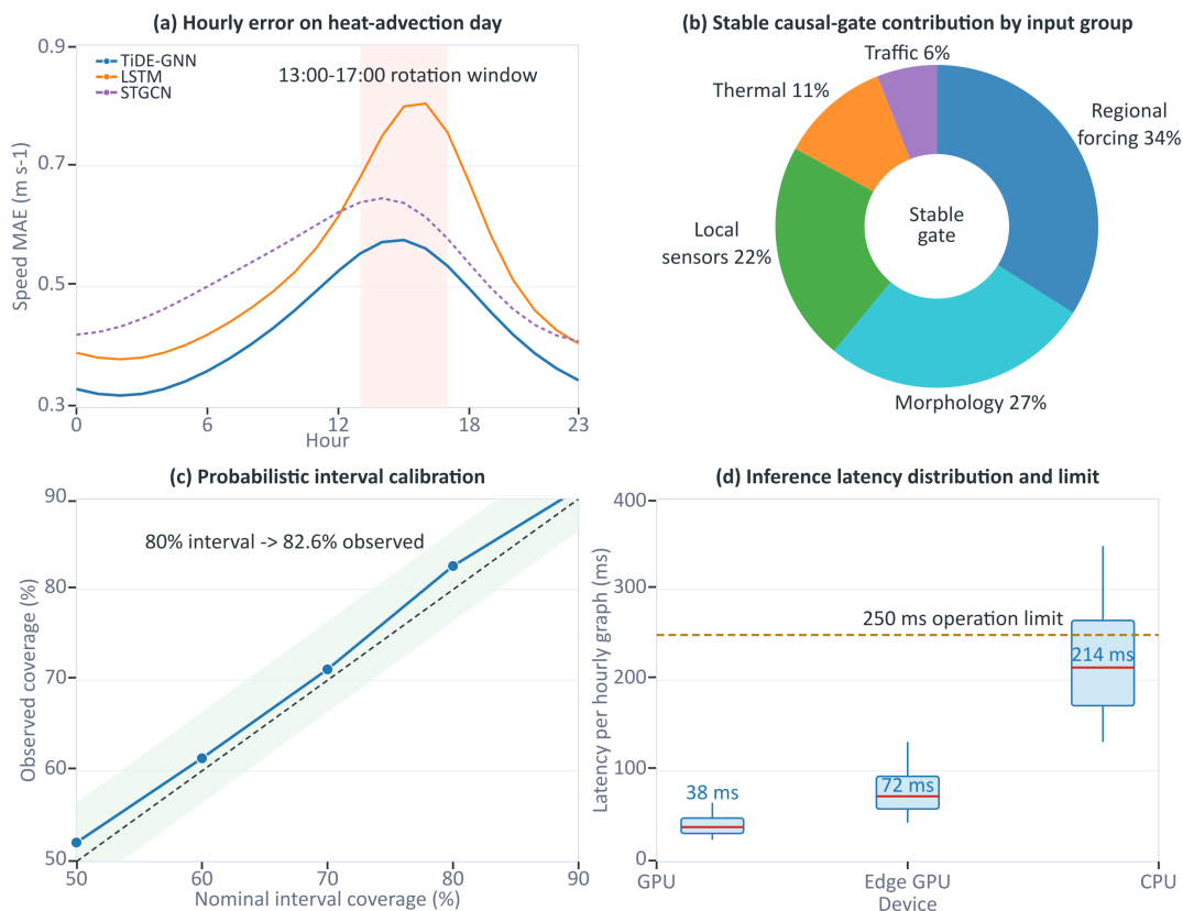
Figure 7. Temporal behavior, causal contribution, uncertainty, and latency: (a) hourly MAE on a heat-advection day; (b) stable gate contribution of input groups; (c) predicted interval calibration; (d) inference latency distribution.
